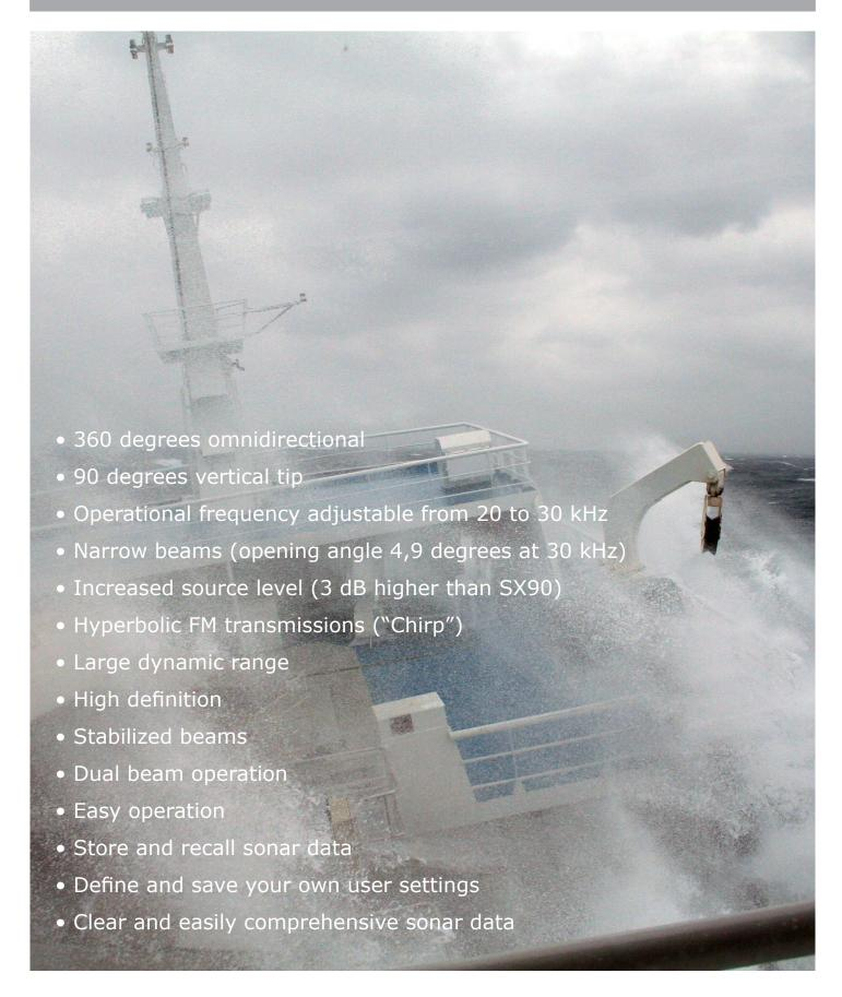
The Simrad SU90 is a long range omnidirectional low frequency sonar. It is designed for medium and large sized fishing vessels, preferably for purse seiners, but it is also well suitable for trawlers.
